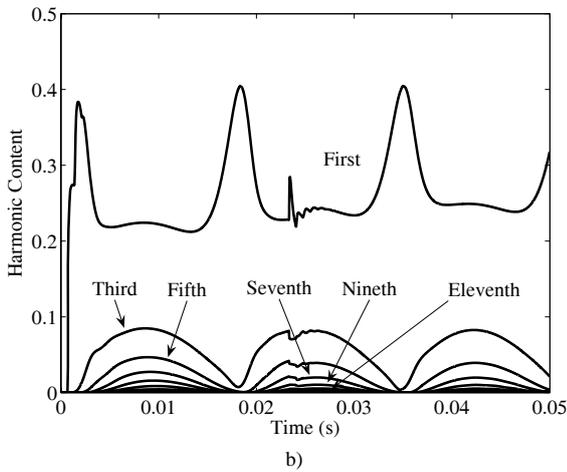
Fig. 7. a) Voltage and its b) harmonic content at bus 4
