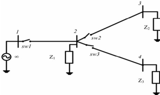
Fig. 5. Network configuration with four buses
