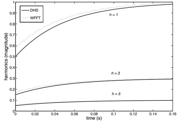
Fig. 2. Harmonic dynamics for time-varying signal
