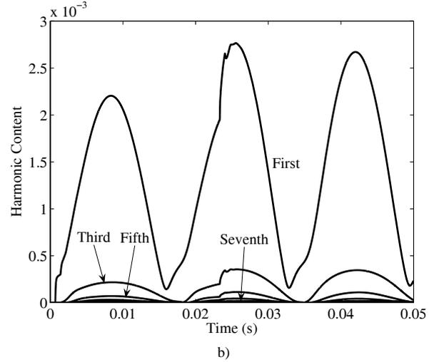
Fig. 8. a) Load current and its b) harmonic content at bus 4
