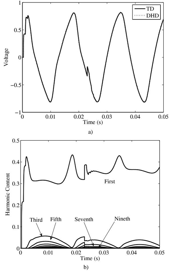
Fig. 6. a) Voltage and its b) harmonic content at bus 2
