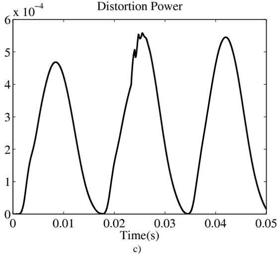
Fig. 9. a) Active, b) Apparent, and c) distortion powers at bus 4
